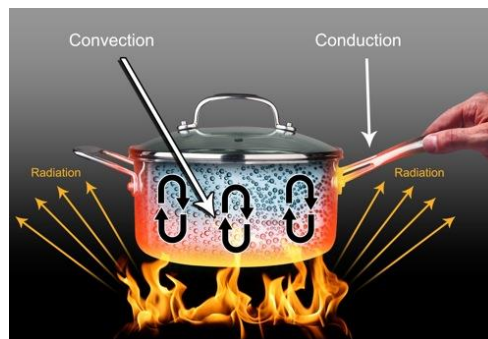
Fig No. 3.1 Modes of Heat Transfer
